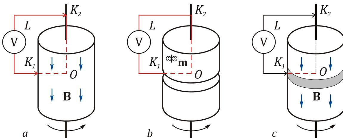
Fig. 5.1. Unipolar generator with a permanent rotating magnet
